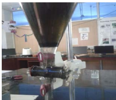
Fig 2-Solution with lead sulfide Quantum dots and 1-Hexane in Separation funnel.
